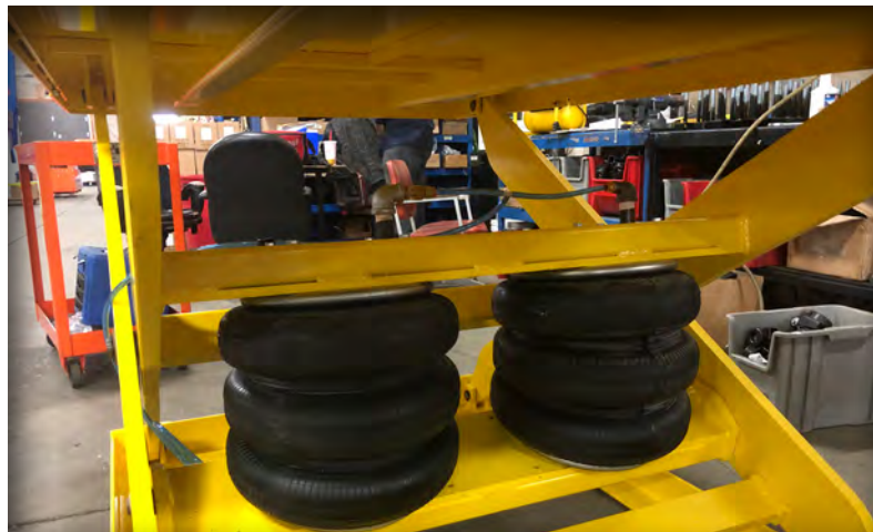
Pneumatic system installed on the above lift table.
