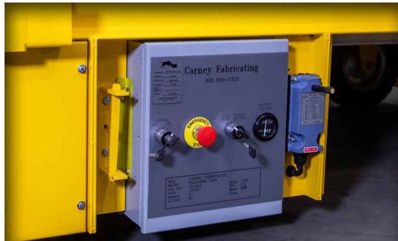
Carney transfer carts include control gauges with E-Stop buttons and are equipped with all safety sensor devices required for ground-level machinery movement
