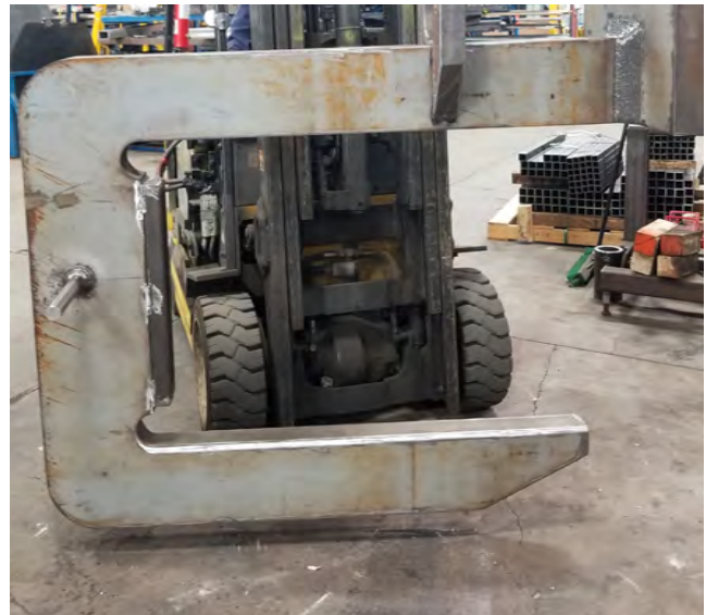
Twenty-five ton c-hook in production before paint
