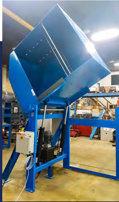
View of product hydraulic components & control panel
