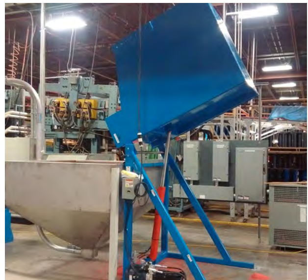
Front loading hydraulic dumper in action
