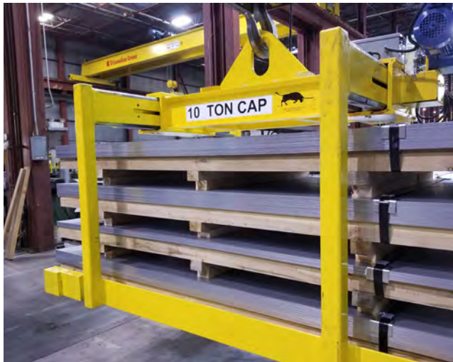
Sheet lifter properly loaded
